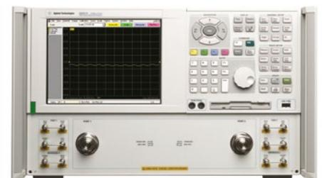
software, capable of handling 300-mm wafers and measuring up to 67 GHz. The laboratory will enable research groups to perform precise electrical measurements on semiconductor integrated circuits (ICs), directly on-wafer, and will be fully supported by specialist applications personnel and measurement consultancy.
